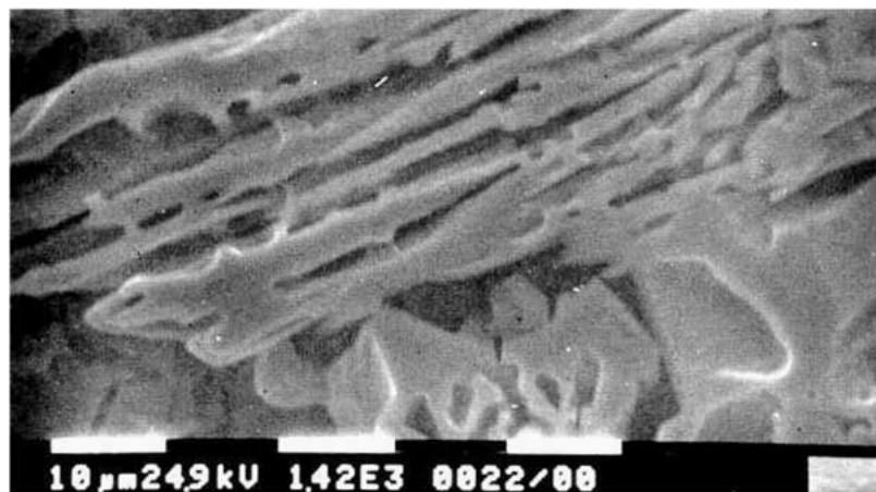
Figure 7 Alloy E, 1.5%C, 14 vol% eutectic carbides. Deep Etching demonstrates that the alloy with the lowest carbon content still has a continuous eutectic carbide network.
