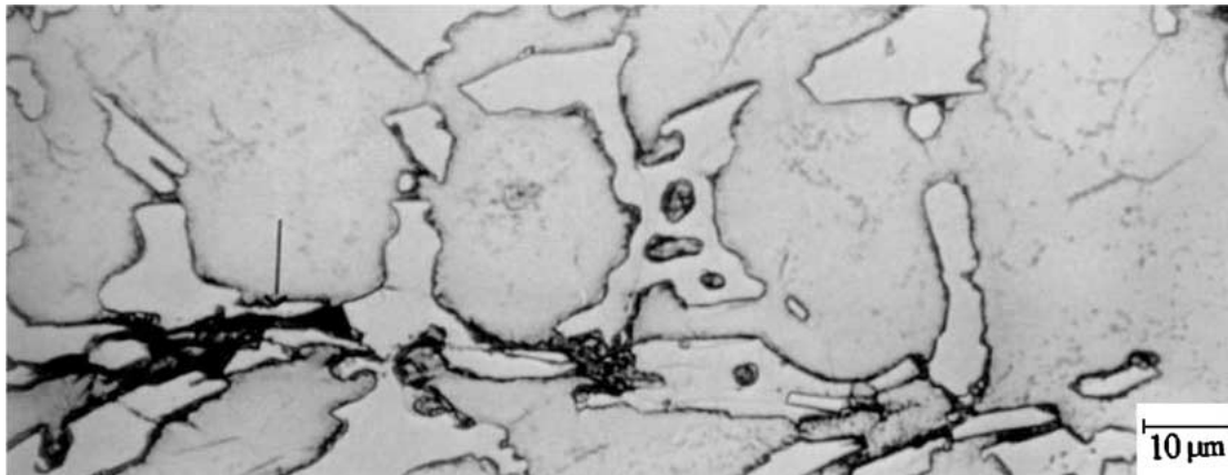
Figure 20 Cracking through the eutectic carbides. The arrow indicates the crack tip.
